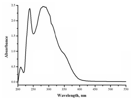
Fig. 1 UV spectrum of Schiff base synthesised from cinnamaldehyde and aniline
